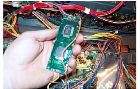
9) This is the Display backside. 3 cables: mid-brown (top), brown and yellow - they'll power your EL-plate from the inverter. CAUTION: The inverter is powering the EL-plate with ~600 Volts, DON'T TOUCH IT when the DSS is powered on!
