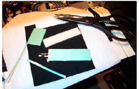
15) Put the old plate to the top of the new plate (both with front side)- new backside is green (or blue) or silver (just as on the old plate). The front sides are white (always!)
