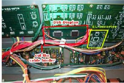
5) This is the Display (red area) and the little plate for the inverter (yellow). 6 screws to be released.
