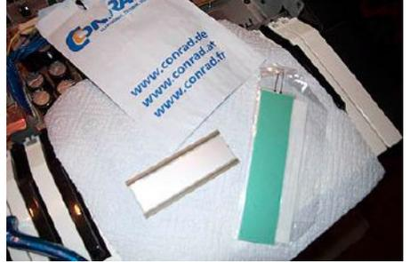
13) Now here's a hint: Fix the "zebras" (the silicon stripes) with the LCD with **super glue (next pic blue)** to the board – but really **FIX** it! The LCD is just on top of the board, no screws etc. You can lift it but if you do so (I did) you're very buys later! The zebras (and the contacts inside them) have to match exactly later again. **IF NOT – check out pic xx, best case: you display will work, worst case: some le\*t\*e\*s a\*e mi\*s\*ng or very worst case: the display will NOT work!**
