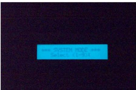
FINAL: This is how it should look like! (After i finally got the zebras matching exactly to the contacts.) Btw: I read about a noisy beep at the Ensoniq ESQ-1 – its the display, if the EL plate does
