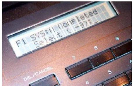
18) Push the new plate (white side to top, colored side down) under the LCD display. Power you DSS ON and check the light. Does it work? ok, Power OFF.
